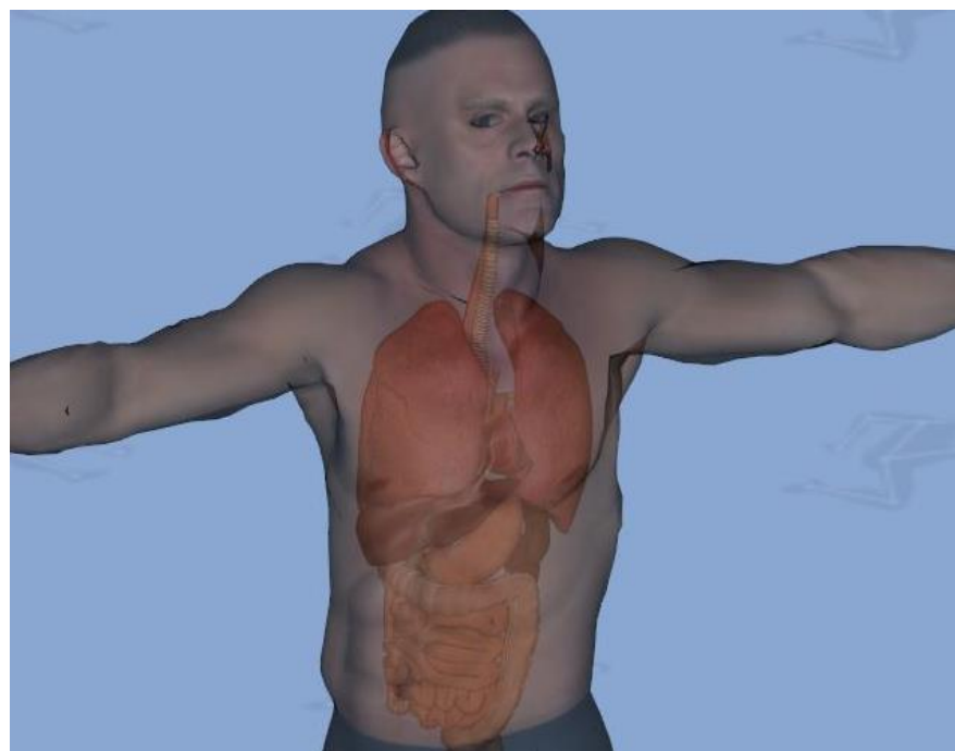
Figure 34: Dynamic model of the lungs deforms to stay within the DHM's skin-mesh in extreme posture
